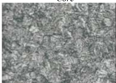
Center hardness: 329 HV
