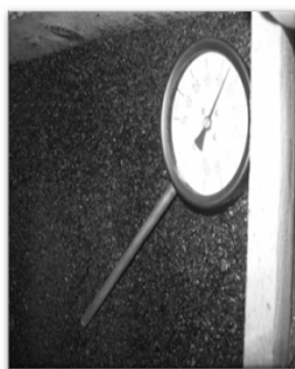
Photo 8, 9 Location of thermometers The asphalt surface The water tank T3
