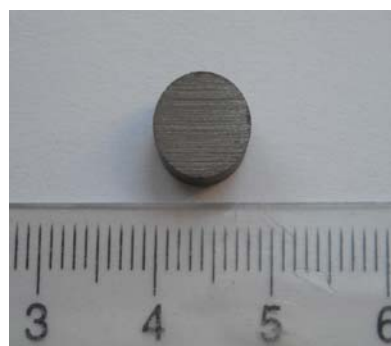
Fig. 4. Aspect of worn surface after the abrasion test
