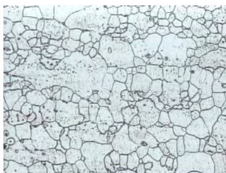
Fig.12. The microstructure of the Al-Zn alloy after quenching in solution and artificial ageing at 150 °C for 6 hours (x100, attack natal).
