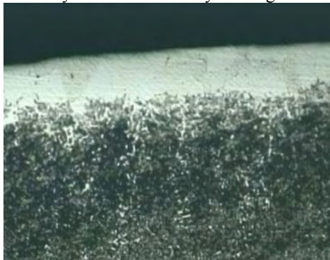
Fig. 8. Nitrocarbured surface layer on the sample R5 (code R), before wear process tests.
