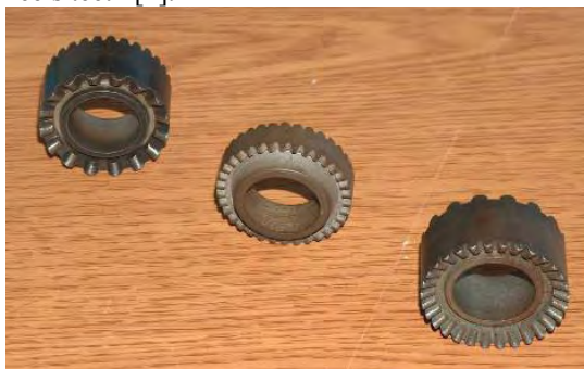
Fig. 5. Sintered satellites from P/M for precessional transmissions.
