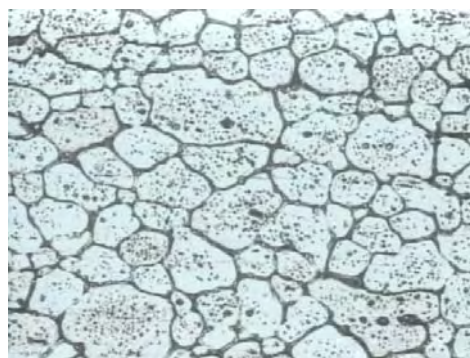
Fig.13. The microstructure of the Al-Zn alloy after quenching in solution and artificial ageing at 120 °C for 6 hours (x100, attack natal).
