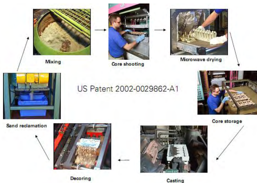
Fig. 1. Castings production using the AWB process.
